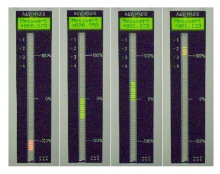
Mode <u>000,002</u> – Green bar from centre of tolerance range (0%) to plus or minus. When the tolerance limit is exceeded, the display is switched to yellow bar from UL (+100%) to plus or red bar from LL (-100%) to minus.
