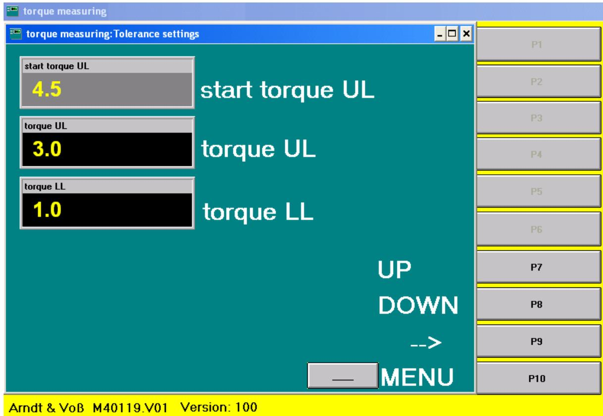
start-torque UL Upper limit for start-torque
