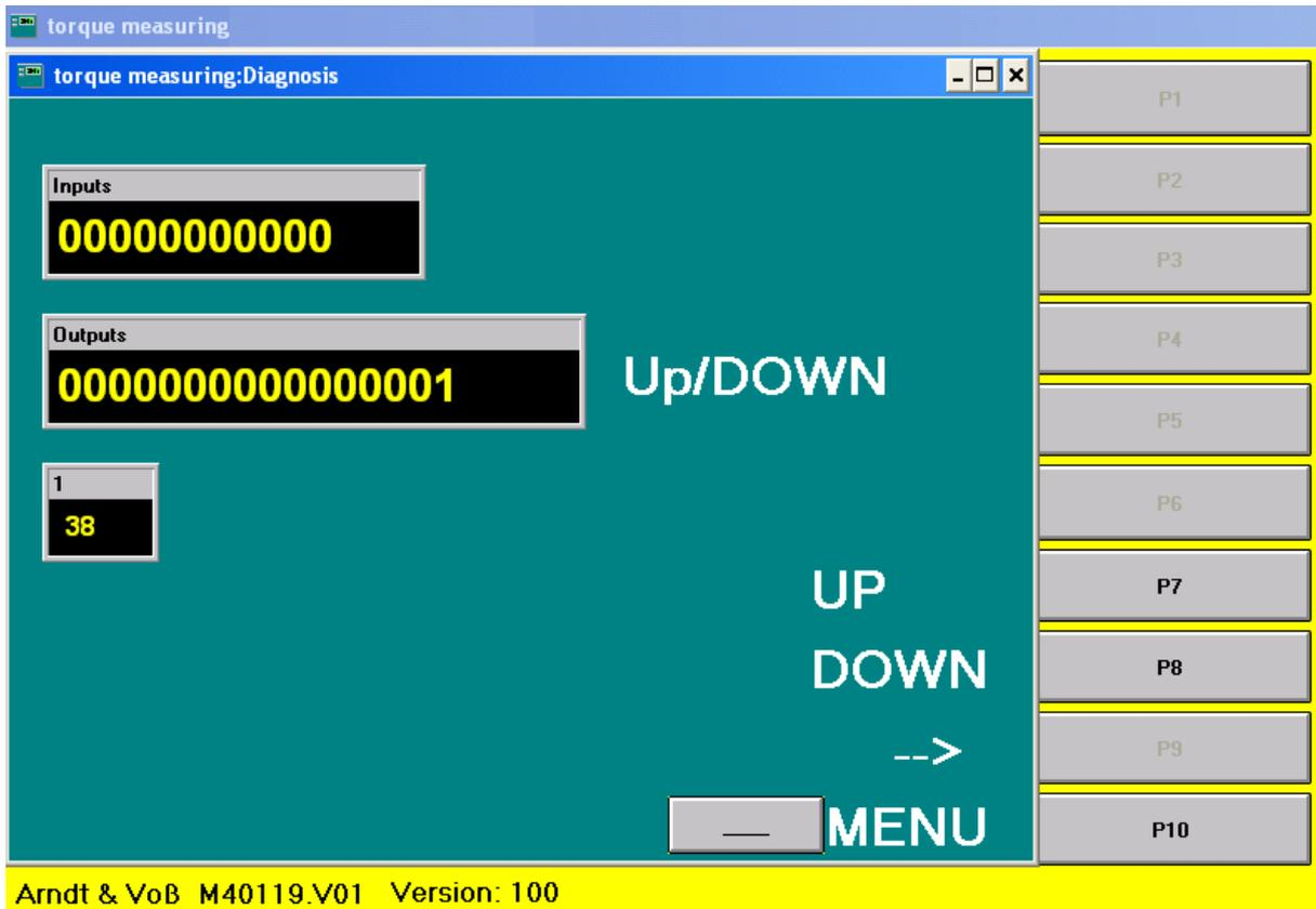
The actual values of the control inputs are shown (1=ON, 0=OFF)
